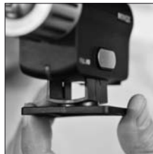
Fig. 7 Mounting the camera: Push the adapter carefully into the mounting bracket
