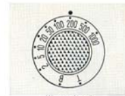
Illustration 5 Shutter Speed Dial (set at 1/200 sec.)
