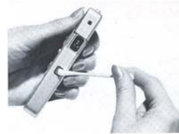
Clean lens window with cotton swab or with a clean linen cloth wrapped around a match or wood stick.
